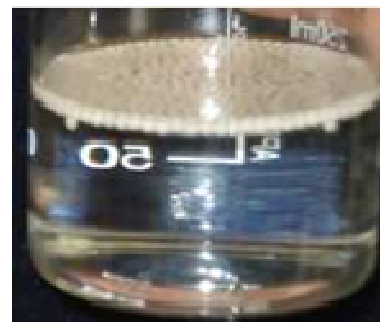
Fig 2: pectin beads floating in simulated gastric fluid without pepsin in a beaker (side view).
