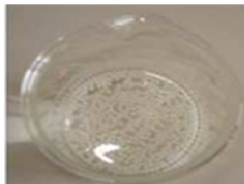
Fig1: Pectin beads floating in simulated gastric fluid without pepsin in a beaker (top view).
