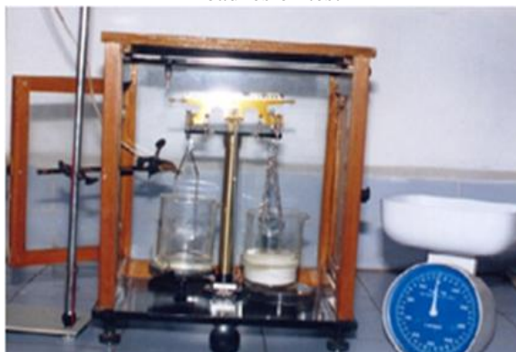
Figure No. 01. Modified apparatus for in-vitro Bioadhesion test
