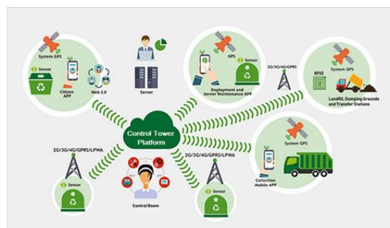
**Figure 3:** Be'ah eco-system which will provide an integrated smart waste management system for optimization of existing collection, transportation, treatment and final disposal of waste operations.
