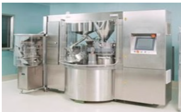
Figure 4: Encapsulation of mini-tablets by Bosch GKF 2500.
