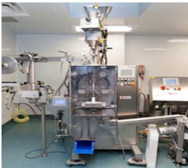
Figure 5: Unit-Dose packing of mini-tablets by stickpack (SBL-50 from Merz System).
