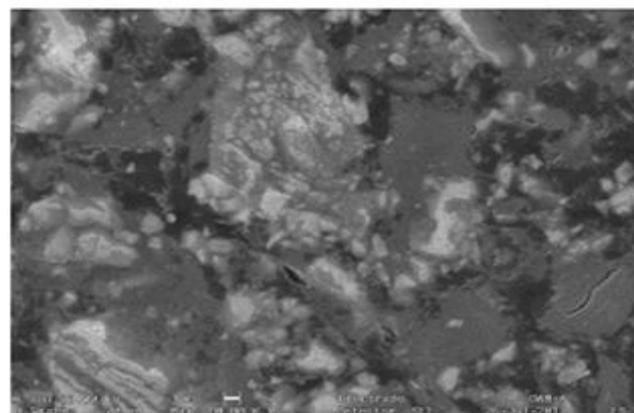
**Figure 4:** SEM micrographs of the electrode, taken with a resolution of 1  $\mu\text{m}$  and an acceleration potential of 20 KV.
