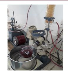
Figure 1: The concentration by rotary evaporation.
