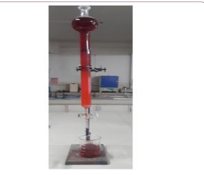
**Figure 2:** Colum chromatographic purification of the prodigiosin solution, this process enhanced the removal of the excess extracting solvent and separated the pure PG from other contamination agents.
