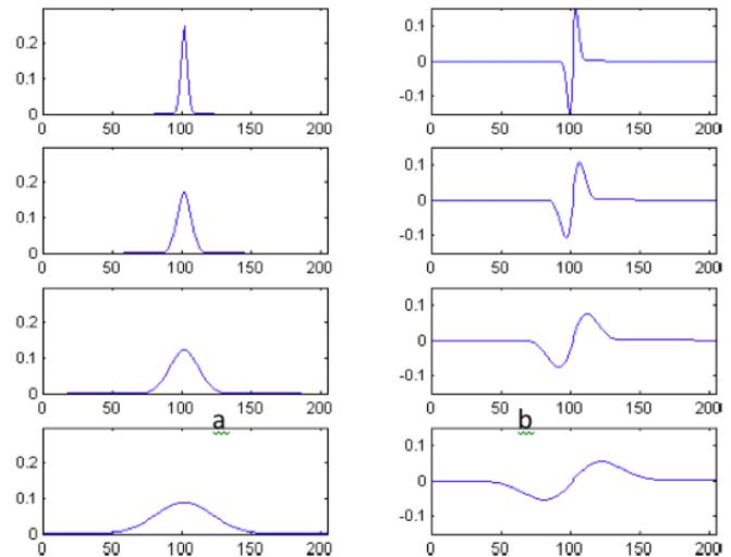
**Fig. 1.** Figure illustrates different filters shape in the Fourier domain, a: real part of the low-pass filters for the scales  $j = 4, 5, 6$  and  $7$ , b: imaginary part of high-pass filters  $\psi$  for the same scale.
