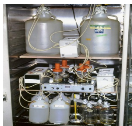
Figure 1 In vitro microbial caries model system.
