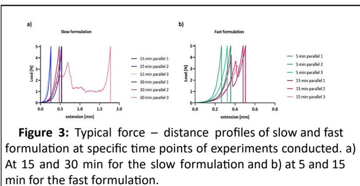
**Figure 3:** Typical force – distance profiles of slow and fast formulation at specific time points of experiments conducted. a) At 15 and 30 min for the slow formulation and b) at 5 and 15 min for the fast formulation.
