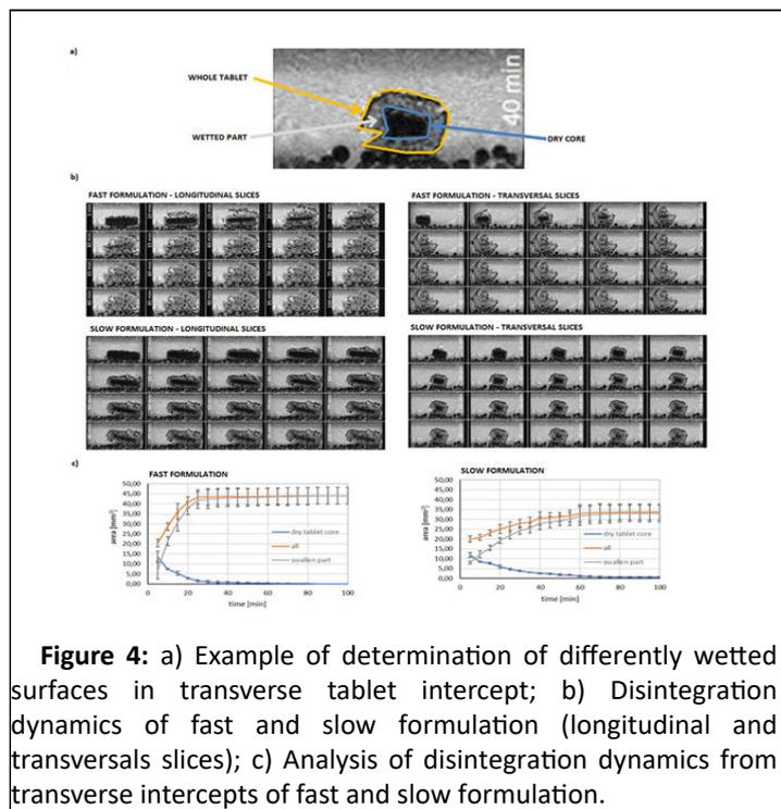
**Figure 4:** a) Example of determination of differently wetted surfaces in transverse tablet intercept; b) Disintegration dynamics of fast and slow formulation (longitudinal and transversal slices); c) Analysis of disintegration dynamics from transverse intercepts of fast and slow formulation.
