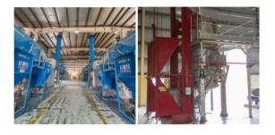
**Figure 2:** An incineration and autoclaving devices in healthcare waste treatment facility.
