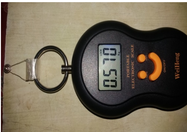
Figure 10 3 mm mouth opening force recorded for syringe made clips with electronic weighing scale.
