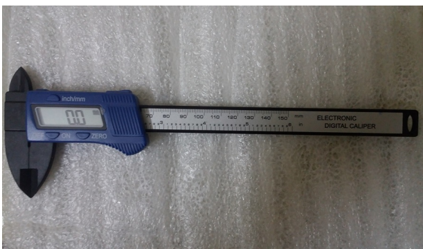
Figure 11 Electronic vernier caliper used to measure clip mouth opening force.
