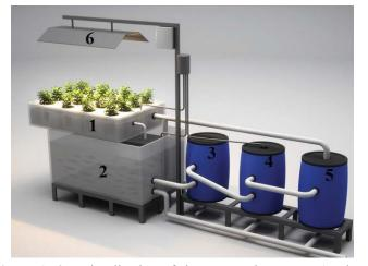
**Figure 1:** 3D Visualization of the aquaponic system. 1: Plants hydroponic tank (raft system) 2: Fish tank 3: Mechanical filter 4: Biological filter 5: Sump 6: Lamp.
