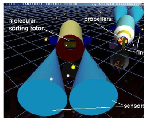
Figure 16: The depicted blue cones show the sensors "touching" areas that triggers the nanorobots' behaviours.
