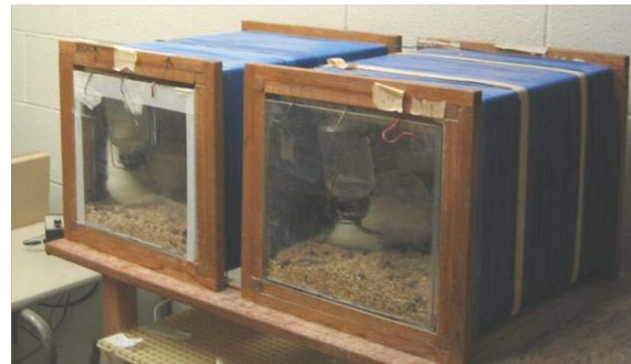
Figure 1 Coils employed to generate the amplitude-modulated 7 Hz magnetic fields.
