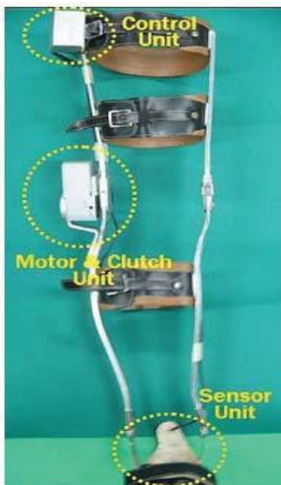
Figure 2 Clutch mechanism in electromechanical SCKAFO is governed by a servo motor [15].
