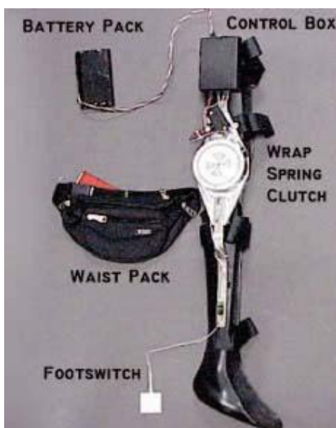
Figure 1 DKBS includes wrap spring clutch, sensors, a microprocessor based control unit and power supply form a rechargeable battery [20].
