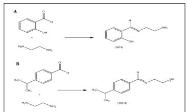
**Figure 1:** Synthesis of Schiff bases. The scheme shows the synthesis of Schiff base I (A) by the combination of salicyldehye 5 mm and ethylene-di-amine 5 mm and the Schiff base II (B) is synthesized by the addition of 4-dimethylamino benzaldehyde 5 mm with ethylene-di-amine 5 mm and the mixture was refluxed at 150°C for 5 h to obtain the Schiff basses I and II.
